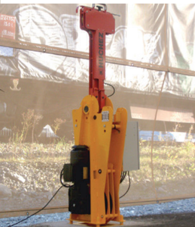
► Innovative solution for rapidly loading and unloading railway carriages (Load: 150 daN, 28 m of textile rope 5 mm dia.).
