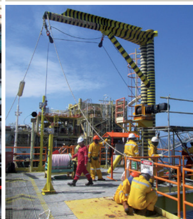
► ATEX lifting winch used on an oil platform. Equipment for zone 2 gas (category 3). Capacity: 2,000 kg and lifting speed: 5.5 m/min on the top layer, 60 m of wire rope 12 mm dia.
