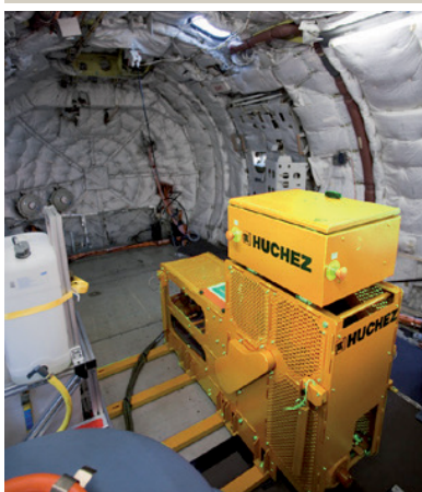
► Autonomous flight test winch for acquiring atmospheric pressure measurements. Load: 140 daN, speed: 30 m/min. © AIRBUS
