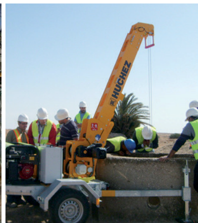
► Well inspection mobile crane. Max. useful load: 140 kg (1 person), max. depth of well: 115 m, average lifting speed: 15 m/min (on adjustable speed drive).
