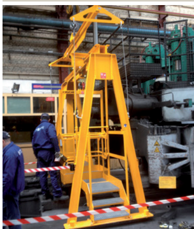
► Gantry crane holding a nacelle used during the maintenance of a rotating laminator. Max. useful load: 240 kg, lifting speed of 5 m/min, max. working depth: 8 m.
