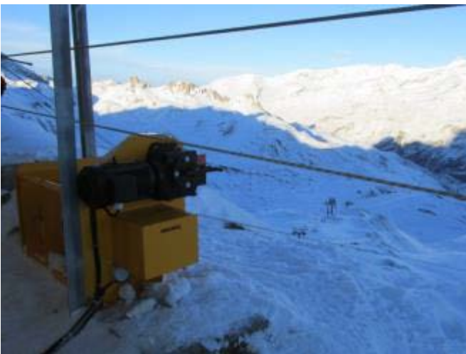
► A winch used to slow a skier's fall when bungee jumping on snow and, once stabilised, zip-lining down to the ground.
