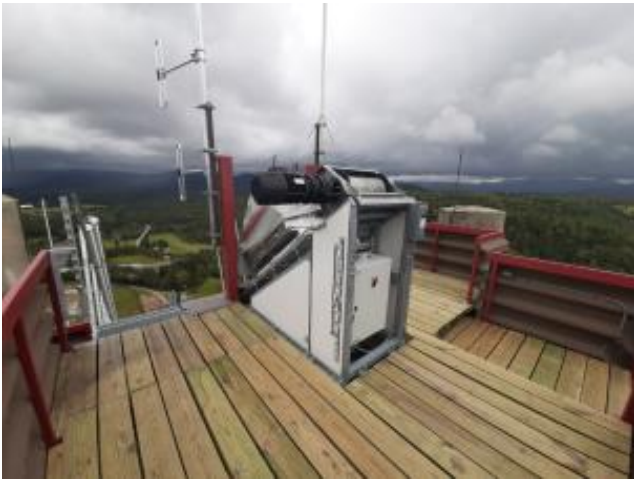
► Electric PL winch on an American ski-jump ramp to lift the machine to remove ice from the rails in which skiers position themselves to the jump.
