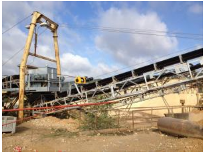
► INDUSTRIA electric winch installed in aggregate quarries to tension conveyor belts.
