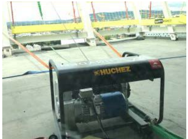
► TRBoxter compact electric winch used to lift heavy loads on the construction site of the new Munch Museum in Oslo.
