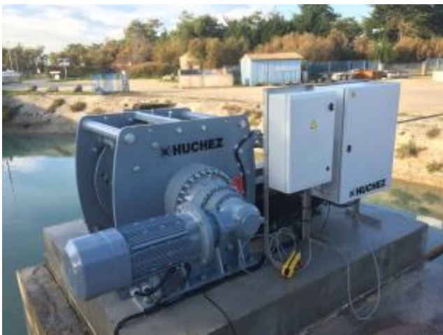
► Electric PL winch on an American ski-jump ramp to lift the machine to remove ice from the rails in which skiers position themselves to the jump.
