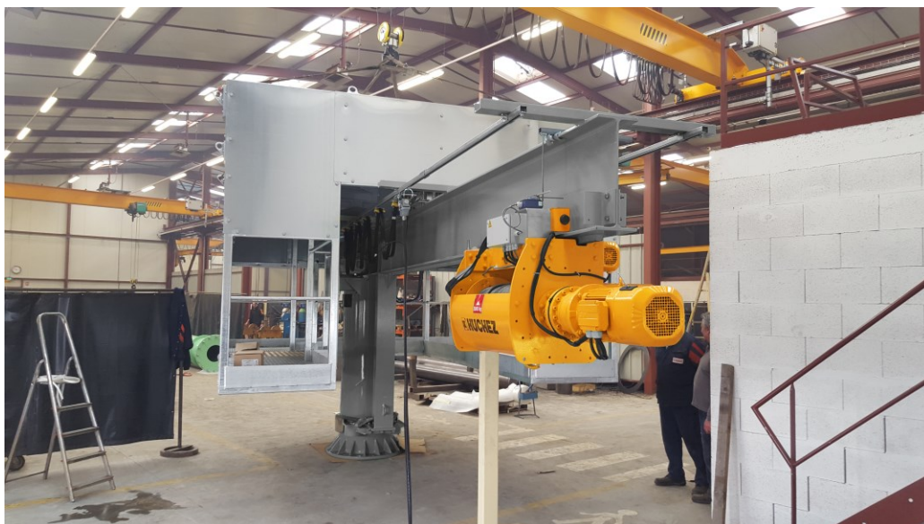
HUCHEZ winch in the workshop during its installation on the jib crane
